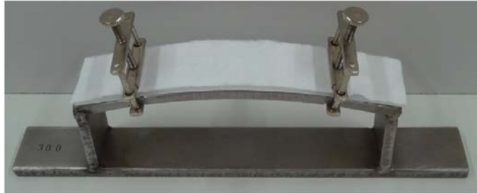
Fig. 1: Test specimens are clamped over a steel template
